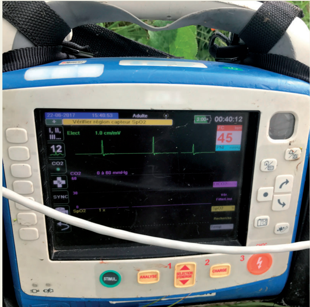
Figure 1 Automated external defibrillator showing a pseudo-pulseless electrical activity cause by an electrical fence in contact with the ground.
